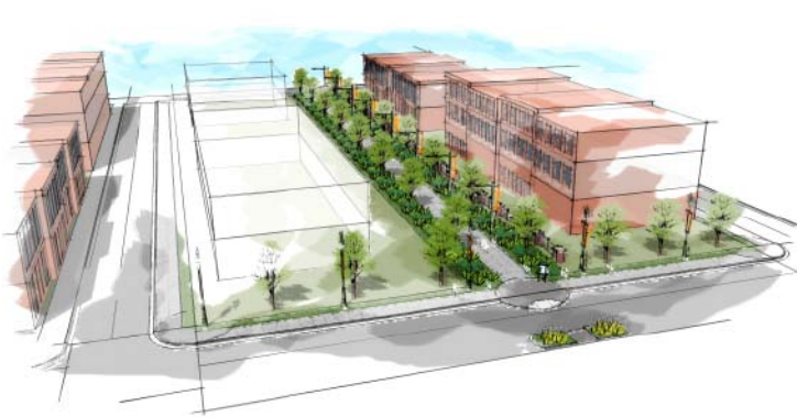
Concept sketch of the proposed Belt Line Greenway showing the trail aligned along the former rail corridor. Enhancements include plantings, lighting, gateways, and crossing improvements.
