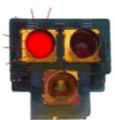
Alternating Flashing Red During Pedestrian Clearance Interval
