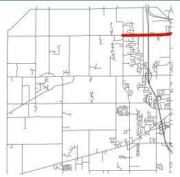
H Avenue from Highway 131 overpass to Drake Road is a two land road with paved shoulders. The road is approximately 30 feet wide, with 12 foot travel lanes and 3 foot paved shoulders.
