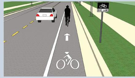
Designated lane for bicycles to travel in the same direction as motor vehicles. Pavement striping, markings and signs are used to identify the bike lane. When riding on a street, a striped bike lane is usually the safest place for a cyclist to ride.
