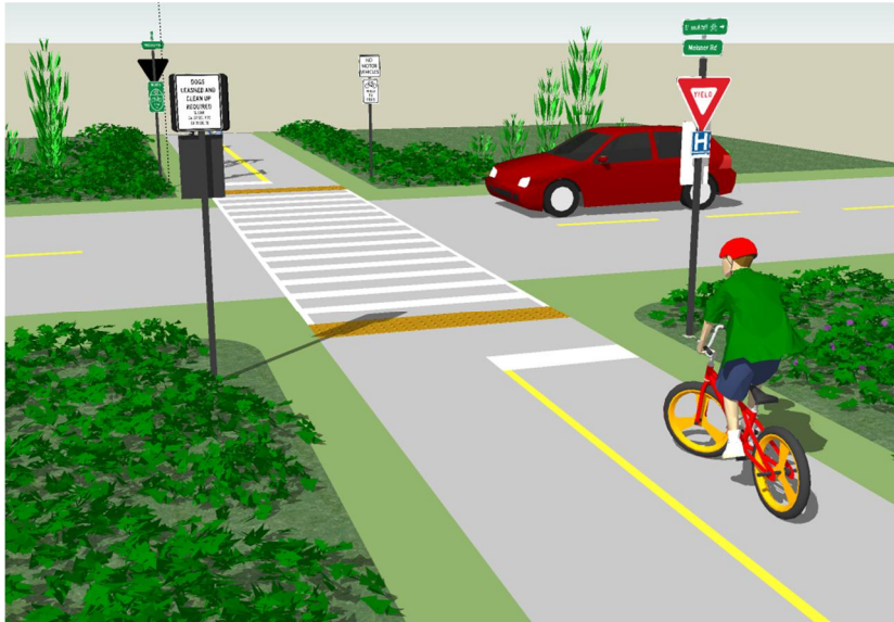
Fig. 5.8C. Trail Signs at Road Intersections Trail View
