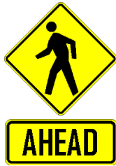
Pedestrian Warning Sign W11-2 and W16-Ahead
