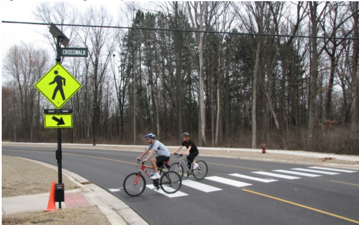
Fig. 5.7H. Rectangular Rapid Flash Beacon
