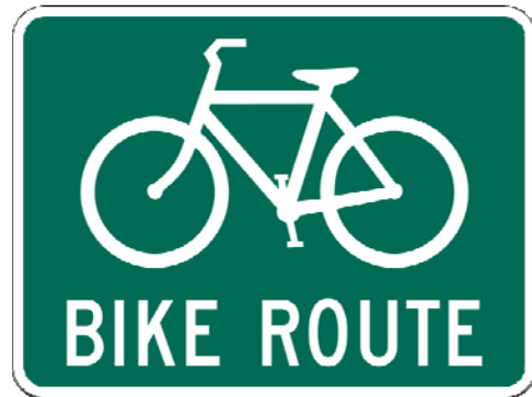
Standard “BIKE ROUTE” sign from FHA’s Manual on Uniform Traffic Control Devices.
