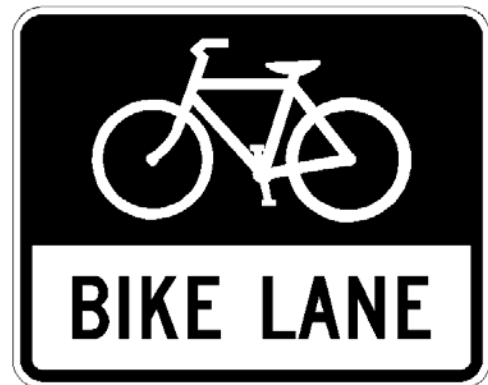
Standard “BIKE LANE” sign from FHA’s Manual on Uniform Traffic Control Devices.
