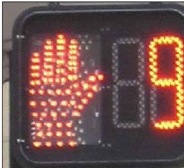
Countdown timers let pedestrians know how much time is left before the traffic signal changes.
