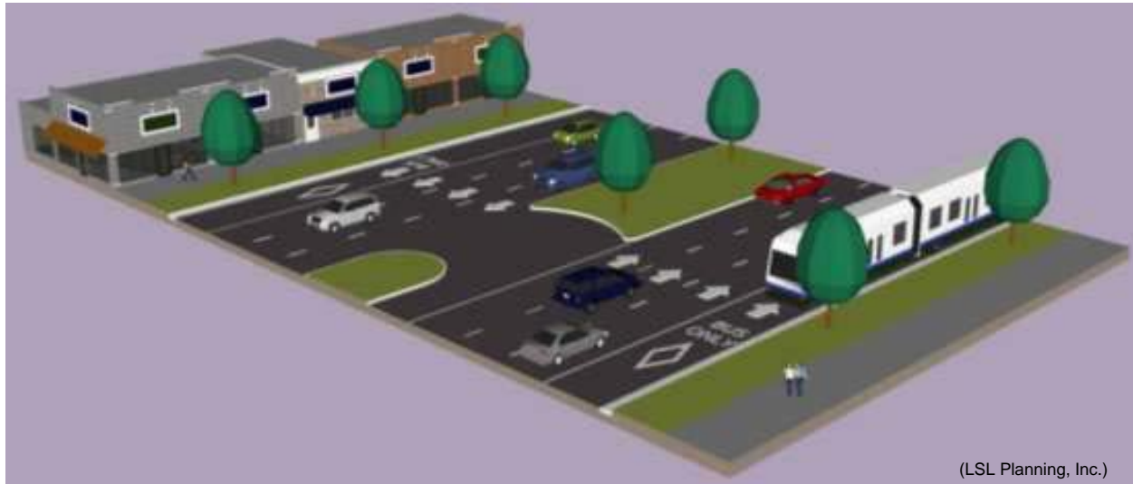
Illustrations of how Woodward Avenue could look if a road diet was implemented. The number of and/or width of vehicular travel lanes could be reduced and the center median narrowed to make room for dedicated transit lanes, or for additional non-motorized facilities like wider sidewalks, dedicated bike lanes, and on-street parking.
